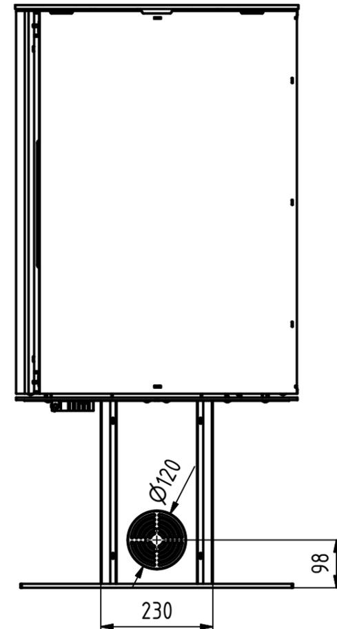
Central - secondary - tertiary AIR CONTROL Central AIR INTAKE - Ø100mm
